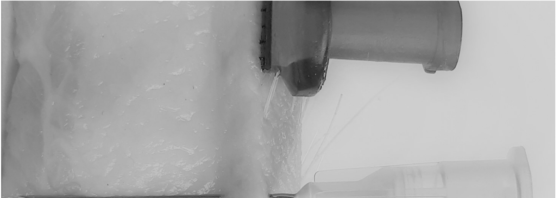
Close-up of a microneedle (top) compared to a hypodermic needle, showing how microneedles are far less invasive
